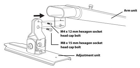
3) Attach the arm plate using a hexagonal wrench (M8) and four M8 x 12 mm hexagon socket head cap bolts.
